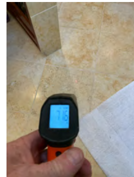
Radiant heating working in master bath.
